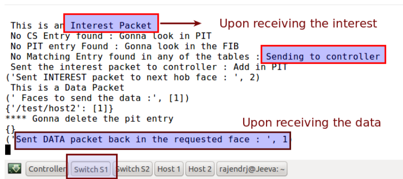
Figure 6.16: OF-ICN and Mini-CCNx comparison : Scenario where some intermediate switches have less forwarding details. OF-ICN host receives content
