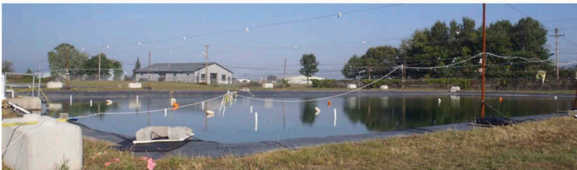
FIGURE 1. Schematic showing the experimental pond indicating positions of the manifold arms, sondes, and pH probes. The pond dimensions were 64.6 m long \times 33.5 m wide. Photograph shows a panoramic view of the experimental pond taken from the south side to indicate the position of the manifold arms.
