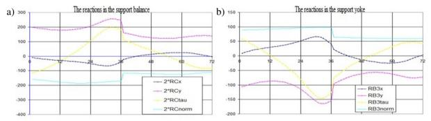
Fig. 3. Behavior of reaction forces (kN) in walking beam support C (a) and equalizer beam support B (b) at initial data: n = 6.8 vol·min<sup>-1</sup>; r = 1.195 m;  $P_B = 80$  kN;  $P_H = 53$  kN
