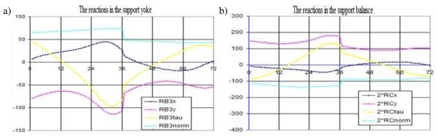
Fig. 5. Behavior of reactions (kN) in pivot joint of equalizer beam B (a) and in support of walking beam C; (b) at initial data:  $n = 6.9 \text{ vol} \cdot \min^{-1}$ ; r = 1.000 m;  $P_B = 60 \text{ kN}$ ;  $P_H = 40 \text{ kN}$
