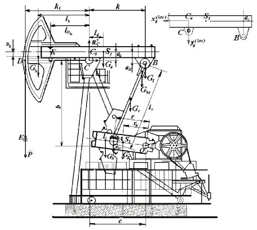
Fig. 1. Converting mechanism of sucker-rod pump power unit
