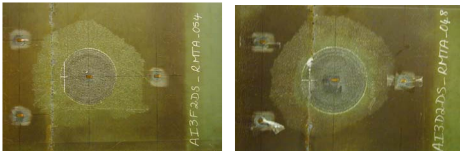
FIGURE 42. FAILURE MODES FOR THE 1/8-inch CORE IMPACTED LARGE FOUR-POINT BENDING BEAMS
