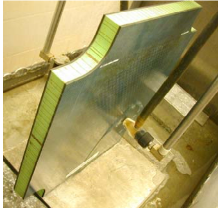
FIGURE 7. WICHITA STATE UNIVERSITY ULTRAPAC SCANNER (C-SCAN)
