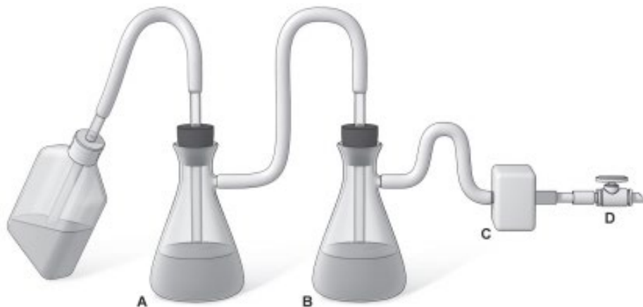
Figure 12. One method to protect a house vacuum system during aspiration of infectious fluids. The left suction flask (A) is used to collect the contaminated fluids into a suitable decontamination solution; the right flask (B) serves as a fluid overflow collection vessel. An in-line HEPA filter (C) is used to protect the vacuum system (D) from aerosolized microorganisms.
