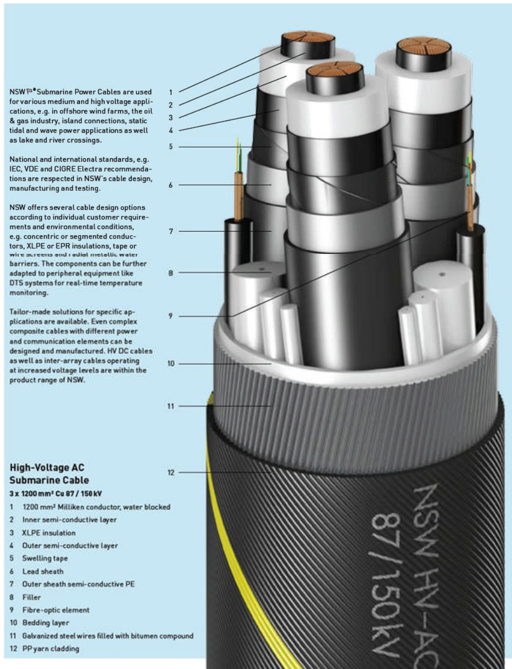
Figure B.1: Typical HVAC Submarine Power Cable: 3 Phase Bundled with Fiber-Optic Elements (Courtesy NSW)
