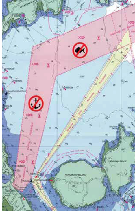
Figure 7.7: Cable protection zone New Zealand
