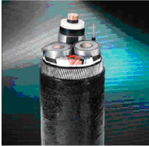
Figure 4.1: Horns Rev Export Cable 170 kV 3 -core XLPE insulated submarine power cable 630 mm 2 Cu-conductor Outer diameter: 194 mm. Weight 79 kg/m
