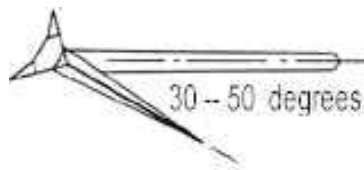
Figure 7.4 Fluke Angle of Typical Ship Anchor
