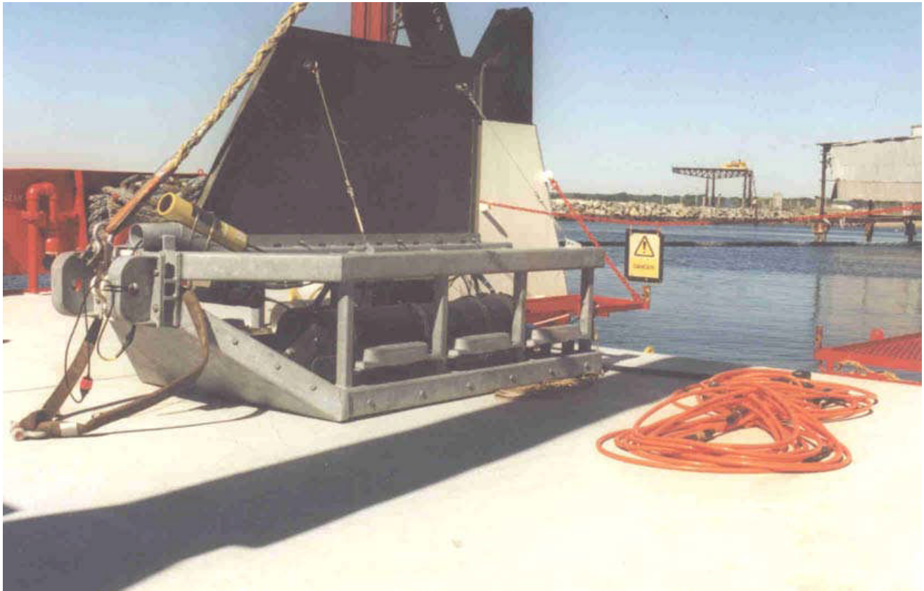
Figure 6.5: Typical Burial Assessment Survey Sled [Ref. 6.9]
