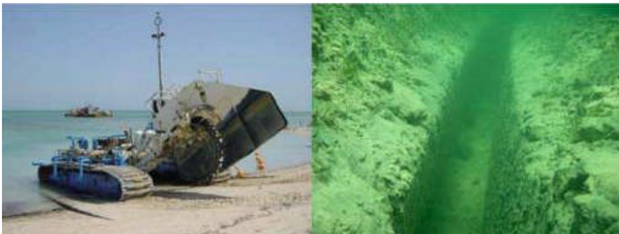
Figure 9.9: Wheel cutter for rocky sea floor Cable trench cut into calcarite sea floor (Courtesy of L.D. Tranvocean) [Ref. 3.36]
