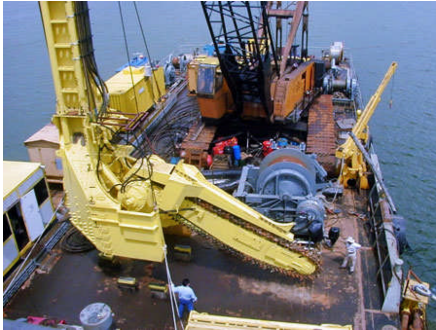
Figure 9.10: Rock saw can reach down 4 meters in soft rock
