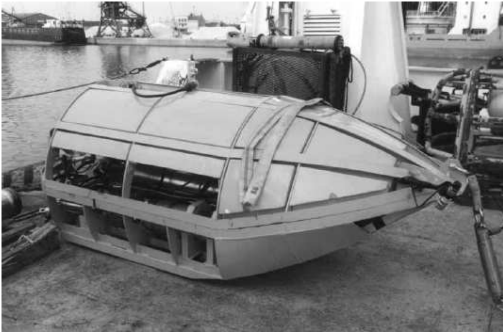
Figure 6.6: GAMBAS – Tow Sled for Seismic Refraction [Ref. 6.14]
