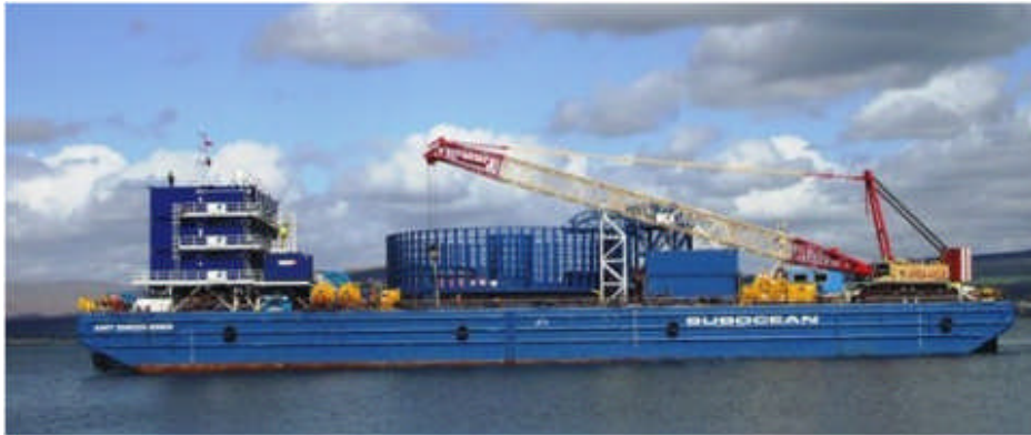
Figure D.3: AMT Discoverer was the cable laying vessel for Rhyl Flats for the inter turbine cables. (Courtesy Anchor Marine Transportation).
