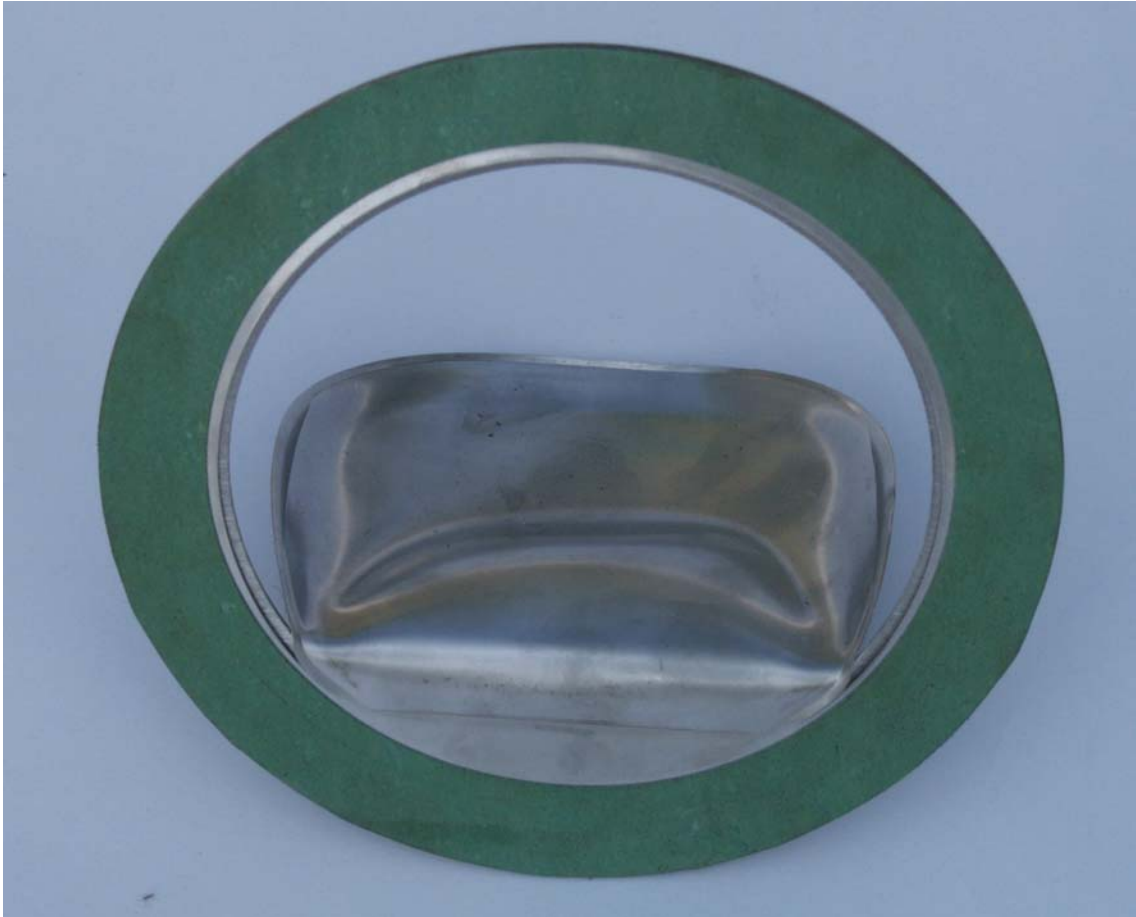
Figure 29 Picture of 4in Steel Burst Disc at Completion of Test
