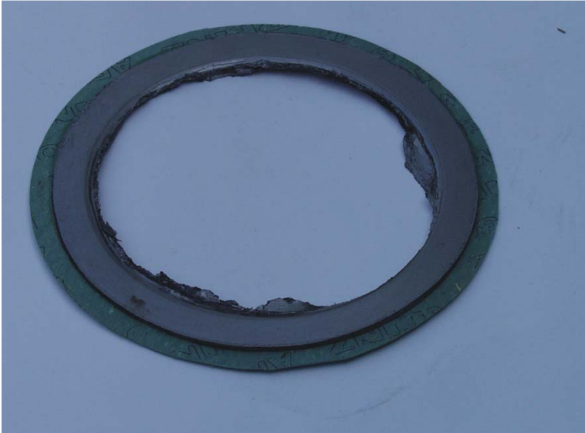
Figure 30 Picture of 4in Graphite Burst Disc at Completion of Test
