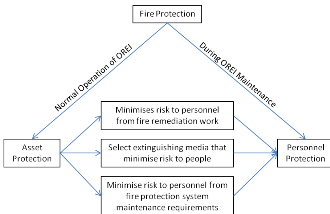
Figure 5: Interrelationship of fire risk and protective measures during normal operation and maintenance.
