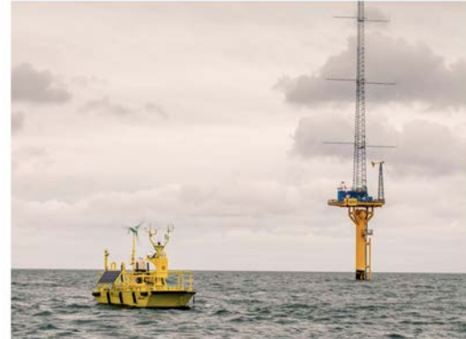
Offshore wind measurements come from ocean buoys, floating lidar* (left) or meteorological towers (right). Photo courtesy of NREL | 11 AXYS Technologies, 35605
