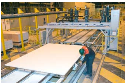
Production line with modular panel laid flat
