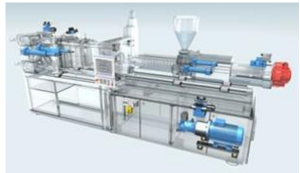
Figure 1: Schematic of hydraulic system in IMM [05]
