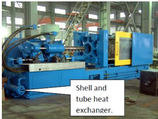
Figure 2: Injection moulding machine using shell and tube type of heat exchangers
