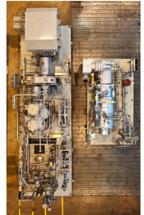
Conventional compressor train
