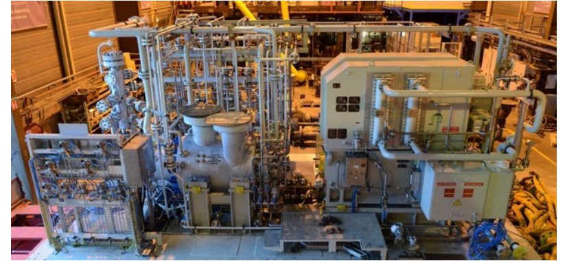
Compressor and high-speed driver in separate casings
