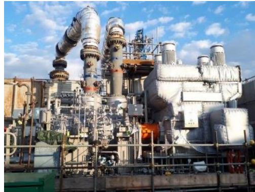
High-speed, direct-drive (HSDD) motocompressor
