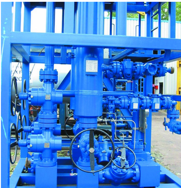
4. SAND FILTER - GATE & PLUG VALVES
