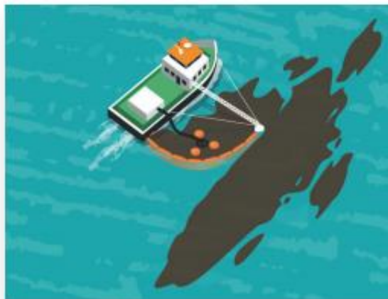
Figure 4 - Example illustration of a single vessel sweep system with jib arm
