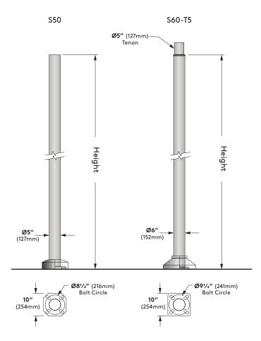
10" x 10" x .75" Base Plate for S50, and a 10" x 10" x 1" Base Plate for S60. Use caution when setting anchor bolts. Bolts must be vertical and centered on dimensions shown. A Ø5" Tenon is required for all poles over Ø5".
