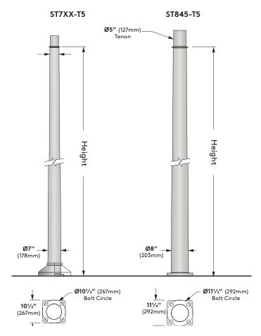
10.5" x 10.5" x 1.25" Base Plate for ST7, and a 11.5" x 11.5" x 1.25" Base Plate for ST845. Use caution when setting anchor bolts. Bolts must be vertical and centered on dimensions shown. A Ø5" Tenon is required for all poles over Ø5".
