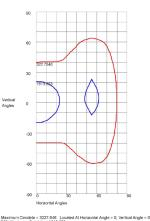
Maximum Candela = 3227.646 Located At Horizontal Angle = 0, V 50% Maximum Candela = 1613.823 10% Maximum Candela = 322.7646
