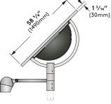
PMO has a 3° angle to allow for drainage. Batteries, Panel, and Hours of Operation requirements to be determined by Selux engineering for every project, please consult factory. Please consult Selux for specific sizing at your geographic location.
