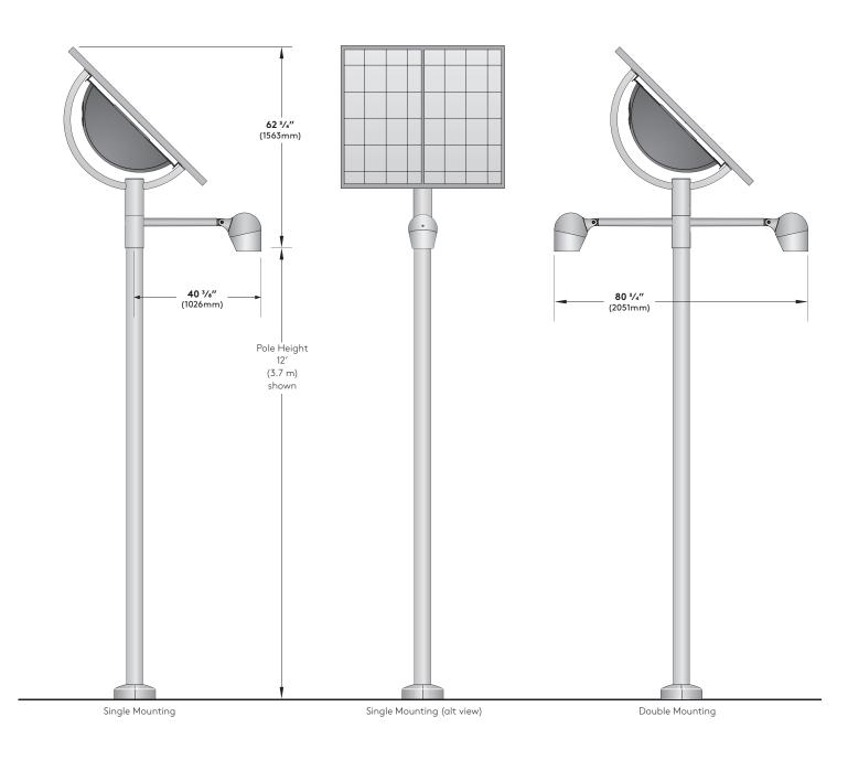
\* = Dimension changes based on panel angle and size configurations. P4 Panel with PM4 (45°) Angle shown. See page 7 for details.
