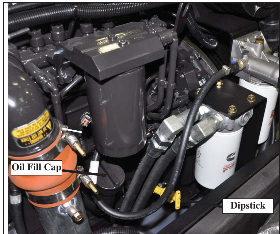
Figure 1-2-2: Oil Fill and Oil Level Check Locations
