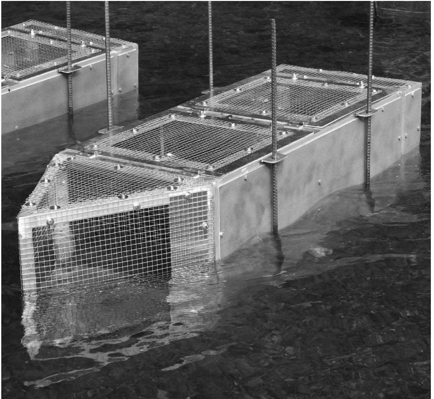
FIG. 3. Flow-through enclosure/exclosures used in field experiments to test for effects of branchiobdellid worms on host crayfish growth (Brown et al. 2012). Flow-through design maintains natural stream conditions while double-walled barriers prevent exchange of branchiobdellidans between enclosed and free-living crayfish (photo credit: BLB).
