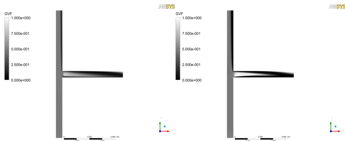
Figure 6.16 Contour plots of volume fraction on mirror plane z = 0 . To the left: CFX Run 2 (with 70 \mu\text{m} bubbles). To the right: CFX Run 3 (with 4mm bubbles).
