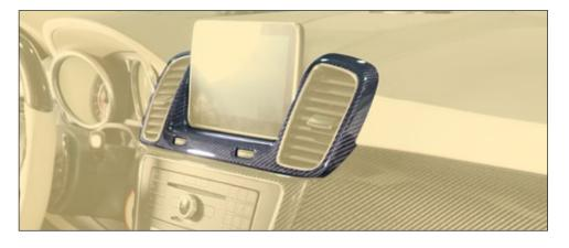
Air vents cover available with carbon and wood O modification only, OE-part required C292 300 011
