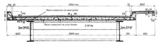
Figure 6: Section through Willerzell Viaduct at Lake Sihl, 1936 (Etzelwerk AG 1934/1935)
