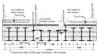
Figure 4: Typical section through railway bridge with rolled beams encased in concrete (Kommerell 1911)
