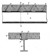
Figure 7: Composite beam (Kahn 1926)
