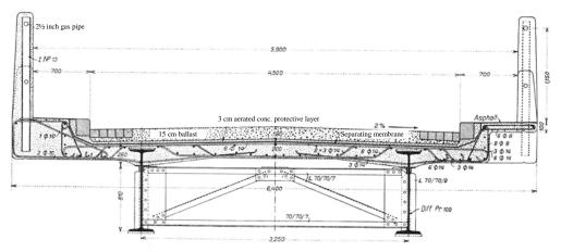
Figure 5: Section through Acheregg Bridge on Lake Lucerne, 1914 (Rohn 1915)
