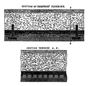
Figure 2: Suspended floor with cast iron joists by Fox & Barrett, pre-1851 (Hurst 2001)
