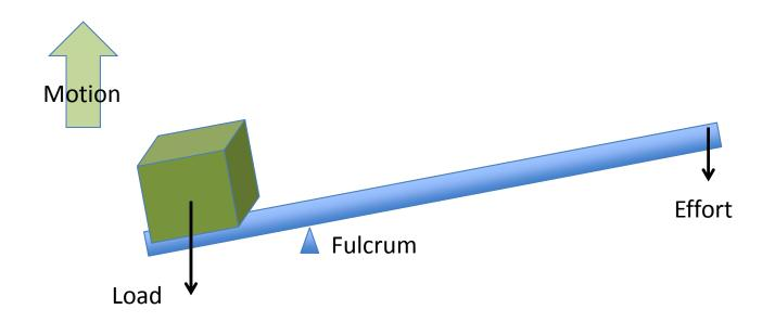
Load: The weight (force) that is being moved Effort: The force being used to move the load
