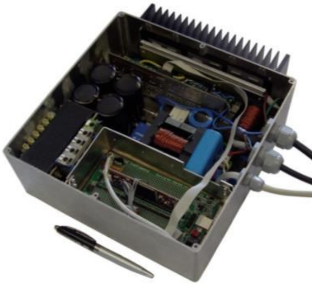
Fig. 14. Developed reconfigurable battery charger prototype.
