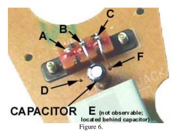
6. Use a pair of appropriately-sized needle nose pliers to remove the capacitor (tubular) shown in Fig.6. Next, remove the wire connecting lug C on the Tone Switch to point F on the PCB. You may need to turn the PCB back over to remove the wire from F by using your soldering iron at that point again. Exercise care.
