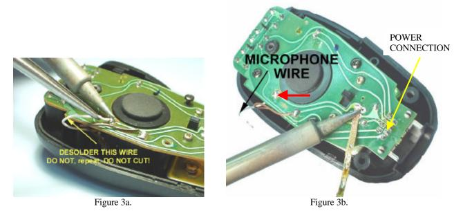
3. Unsolder (see Fig. 3a) the white wire (from the microphone element) that is connected to the PCB at the location indicated by the red arrow in the Fig. 3. Next, using the supplied solder wick, remove the solder on the pads located as shown in Fig. 3b.
