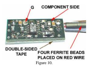
10. Figure 10 shows the One BIG Punch unit. First, remove the paper from the exposed side of the double-sided tape identified in Fig. 10 and keep the exposed tape from touching anything until the next step. The four ferrite-beads will be placed on the red wire in Step 12.
