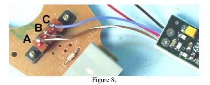
**.** 8. With the One BIG Punch unit positioned as shown in Fig. 8, solder the brown wire with the white trace to lug A on the tone switch and the blue wire to lug C.
