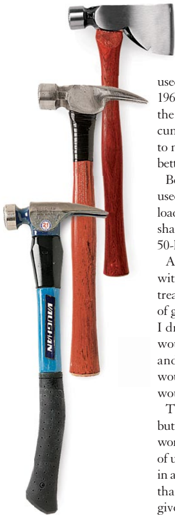
Evolution of the framing hammer. Because the traditional 16-oz. hammer wasn't adequate, some carpenters started framing with Plumb's long-handle 28-oz. rigging hatchet. When they tired of the occasional bloody forehead, carpenters got local welders to cut off the blade and attach a pair of straight claws. The design lives on in hammers such as Vaughan's new Blue Max.
