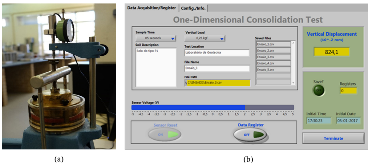
Fig. 4 – (a) Analog and Digital Experimental Setups; (b) Main Window of the developed application
