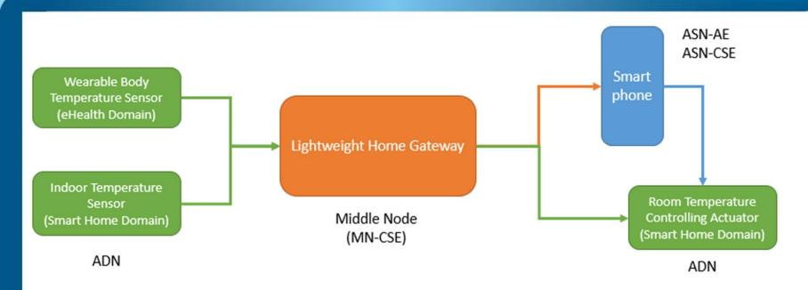
Scenario: The body temperature measurements are processed at the MN. If fever is deduced, a notification is sent to consumer mobile devices. The MN polls the indoor room temperature and provides an option to the person to set a comfortable room temperature through actuation. This smart living scenario combines the elements from both the Smart Home and eHealth domains
