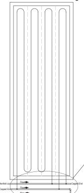
Long manifolds are installed perpendicular to the floor joists. To ensure balanced flow through each circuit, a reverse return method is recommended. A reverse return manifold requires a third copper line to be installed. This extra line allows each circuit to "see" the same total manifold length, thus creating a balanced system.
