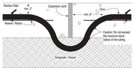
Onix routed below expansion joint into subgrade.
