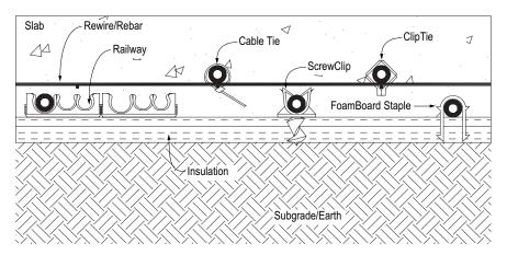
Various tube fasteners for slab applications.
