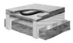
Sandwich applications mimic Staple-Up™ in almost every way except one. In a Sandwich application, the Onix tubing is placed on top of the subfloor instead of beneath. Sleepers are installed every 8" or 16" on center, depending on the floor construction and floor covering requirements. These sleepers mimic the function of the joist in the main floor, aiding support for the upper subfloor that will be added prior to the finished floor.
