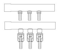
3. 1"× 1/2" × 1" Reduced T-Fittings can be soldered together forming a complete manifold. Onix Barbs are then soldered into the 1/2" fittings.
