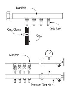
the Onix onto the first barb of the supply manifold, making sure the tubing covers the entire fitting. If the Onix is difficult to push onto the barb, lubricate the end of the Onix with some water.
