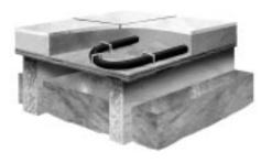
Some construction details call for a Thin Slab, or a lightweight concrete, to be applied above the subfloor. These applications offer increased sound quality to a room and an increased thermal mass to the radiant heating system. In some cases, thin slabs are used to act as a fire-stop from floor to floor.
