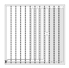
This illustration shows how to "pick up" a bay when the previous circuit terminates mid-run. The second circuit loops back down the open bay from the far end. The remainder of the circuit is installed in the same fashion as the first circuit.
