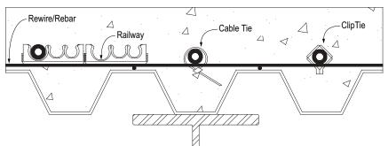
Various tube fasteners for steel deck slab applications.
