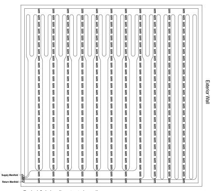
Typical Onix banding at exterior walls.
