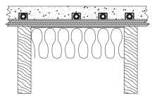
Onix tubing stapled down to the subfloor with paper faced batt insulation located below in the joist cavity. Since no foil facing is used, the insulation has to be installed against the subfloor.
