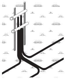
After the concrete is poured and just before the interior walls are installed, the rebar may be cut to free the manifolds. The manifolds can then be moved if necessary, to fit the actual wall construction. Make sure to leave plenty of slack in all Onix circuits (2–5 ft. is recommended). A Watts Radiant manifold box can be used to secure the manifolds within the new wall. Watts Radiant SnapClips and StrapDowns can be used to organize Onix coming from the floor and into the wall.
