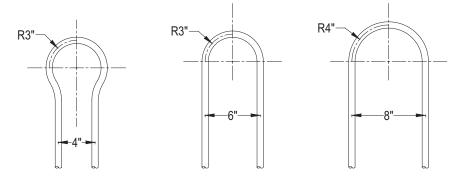
Typical bend radii for 3/8" diameter Onix. Larger diameter tubing will require larger bend radii.
