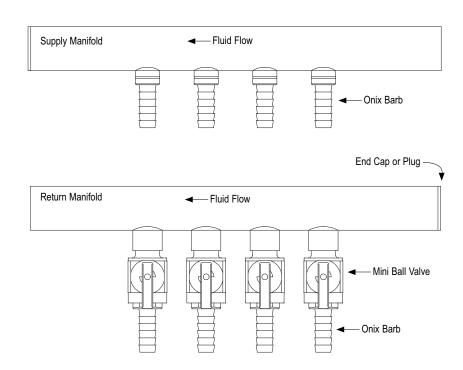
Typical Copper or Tubular Brass Manifold Pair.
