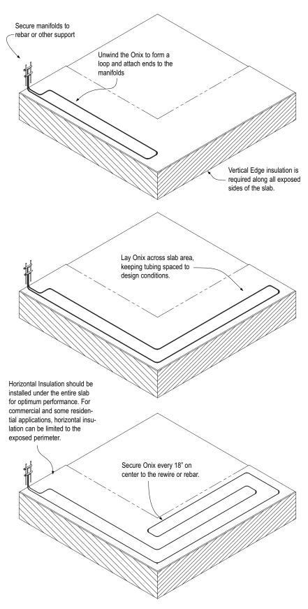
Typical slab installation. Onix is installed using a double serpentine pattern.
