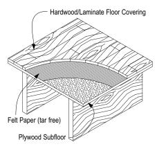
Typical hardwood installation sequence over a frame floor
