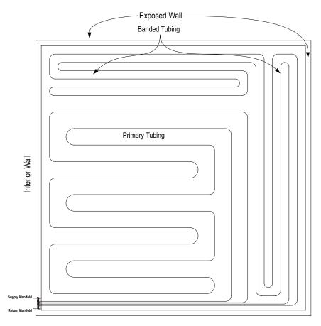
Typical slab tubing layout.
