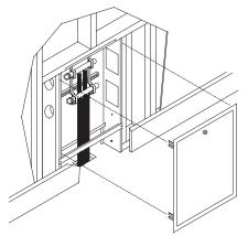
Metal Manifold Enclosure located in wall.
