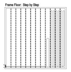
This illustration shows a serpentine layout with a banded area running parallel to the exposed wall. The banded area is spaced at 4" o.c.
