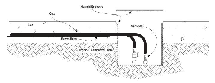
Make sure to leave plenty of slack in all Onix circuits (2–5 ft. is recommended). A Watts Radiant manifold box can be used to secure the manifolds within a structural wall. Watts Radiant SnapClips and StrapDowns can be used to organize Onix coming from the floor and into the protective enclosure.
