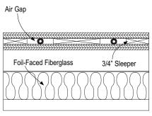
Joist side view showing Sandwich application using foil-faced batt insulation.
