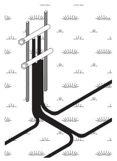
port the manifolds in such a way so they are not damaged during the concrete or paver installation.
