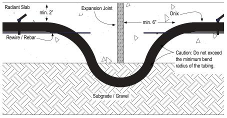
Onix routed below expansion joint into subgrade.
