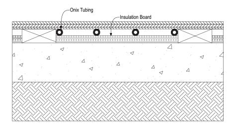
The same techniques are used when installing a Sandwich application over a slab. The use of an extruded polystyrene (Dow® Blue Board®) is recommended for this application.
