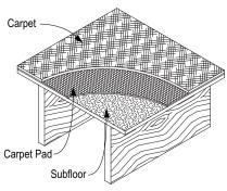
Typical carpet and pad installation sequence over a frame floor.
