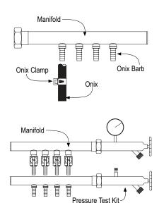
and will tend to cause an imbalance in the fluid flow. Some tubing may be removed from this last circuit as long as the remaining length is within 10% of the existing circuits. For example, if 200 ft. lengths were installed, the last circuit can be cut to a length of 180 ft. and still maintain a balanced system. If more than 10% is in excess, run the remaining tubing along an exposed wall or in other areas of the zone.
