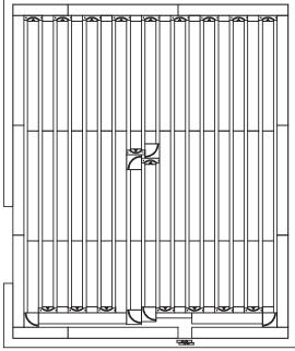
Step 3: Install Sleepers and bend supports
