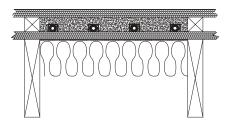
Onix tubing stapled down to the subfloor with paper faced batt insulation located below in the joist cavity. Since no foil facing is used, the insulation has to be installed against the subfloor. A lightweight concrete filler is used between the sleepers for added sound quality and increased thermal mass.
