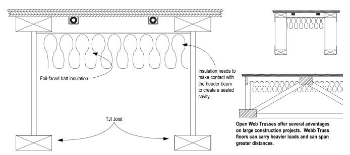
Typical TJI (Truss Joist International) cross-section.
