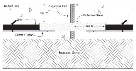
Onix sleeved at expansion joint with foam insulation or PVC conduit.
