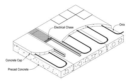
Typical Slab over Precast application. Insulation location and fasteners are variables depending on the structural requirements of the total mass. Consult with the structural engineer before choosing an insulation or fastening method.
