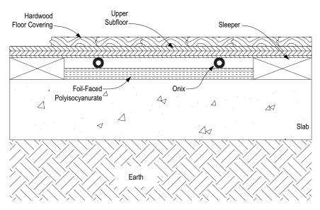
The National Hardwood Council allows the hardwood to be installed directly on top of the radiant tubing. However, it is advised to first install a subfloor over the radiant system to help protect the tubing from nails and other attachment devices.
