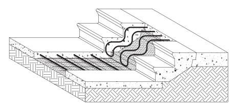
Onix installed running perpendicular to the step. When running perpendicular to the step, make sure there is enough room to make proper bends between the riser and tread and still maintain the minimum coverage requirement.
