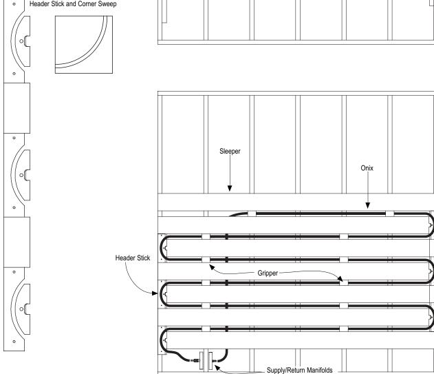
SubRay Sleepers are installed across the studs or joists with Grippers installed every fouth stud or joist to keep the Onix in place.
