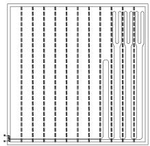
This illustration shows a serpentine layout with a banded area running perpendicular to the exposed wall. The banded area is spaced at 4" oc.
