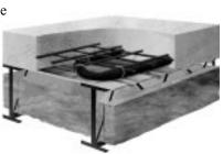
Use a foil-faced insulation for this application, with the foil facing up, and a 2" minimum air space between the foil surface and the steel deck.
