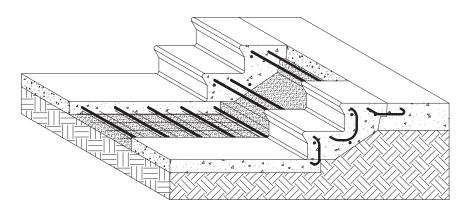
Onix installed running parallel with the steps. An additional run of Onix may be installed in the riser of the step to help increase melting along the outer edge.
