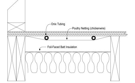
Poultry netting (chickenwire) is used to support the Onix. A foil-faced batt insulation is used below the Onix with a two inch air gap, foil facing upwards.
