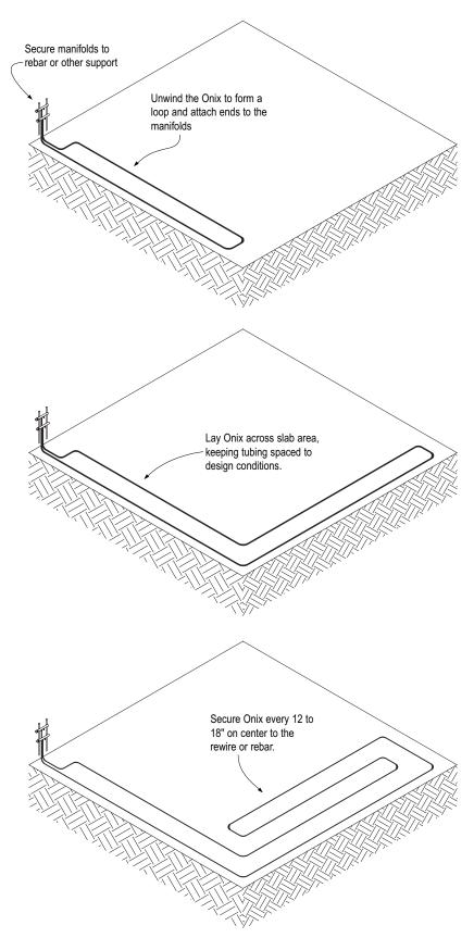
Typical slab snowmelt installation. Onix is installed using a double serpentine pattern.
