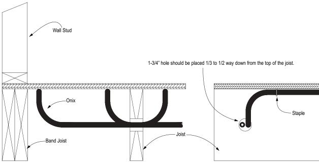
Onix routed through joist in Staple-Up application.
