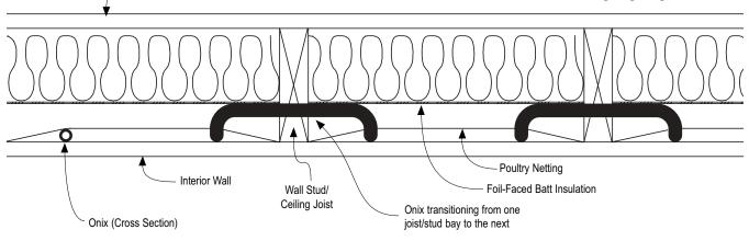
Cross section of a wall or ceiling application using poultry netting (chicken wire).
