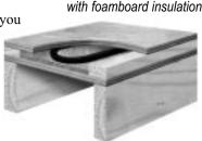
Install a high-temperature foil-faced foamboard insulation, such as Thermax<sup>II</sup> or equivalent, between the nailers. It is very important to carefully select the correct nailer and foamboard thickness, so that the Onix maintains continuous contact with the underside of the upper floor or subfloor, but isn t crushed or deformed.
