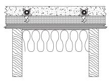
Board insulation is used to isolate the thin slab from the subfloor below. ScrewClips are used to secure the Onix to the foam insulation board. Additional insulation may be added below, in the joist cavity, for an increased R-Value.
