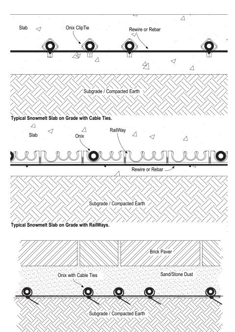
Typical Snowmelt Brick Paver with Cable ties.
