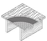
Tile and other stone floor coverings are the most efficient to use over a radiant system. The more conductive the floor covering the lower the required supply water temperature.
