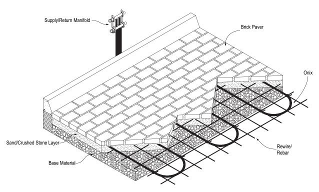
Onix installed in a sand and brick paver application.
