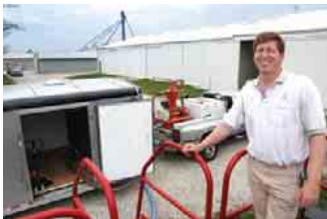
The brothers designed a planter tender based on an enclosed trailer to stay out of the wind and weather when mixing talc or graphite with seed. The 102-inch-wide trailer handles two pallets side by side. They empty bagged seed into two bulk hoppers mounted in the front of the trailer; a grain vac system delivers the seed to the planter hopper.
