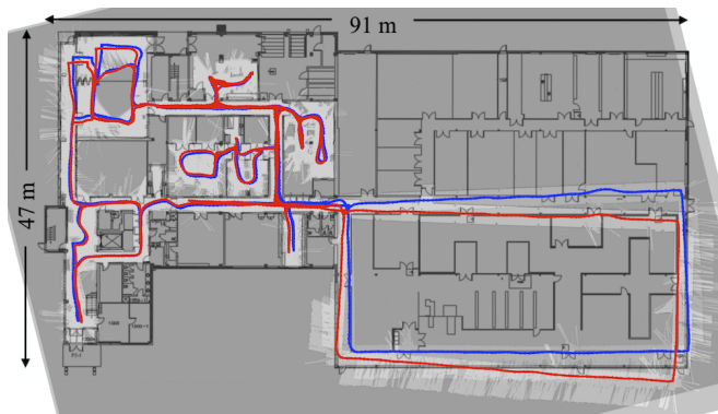
Fig. 11. Global maps with (blue) and without (red) T . The maps are manually superimposed over the actual plan of the building.
