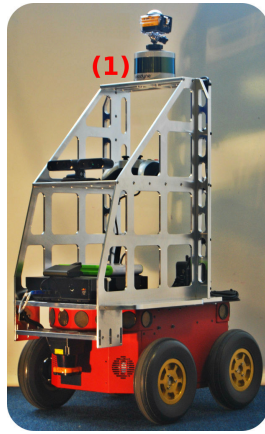
Fig. 6. Robot equipped with (1) a Velodyne VLP-16 3D LiDAR used for dataset collection.
