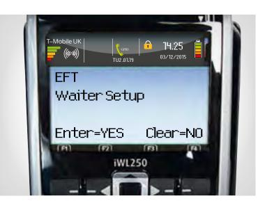
4 Press the button to continue to waiter setup.
