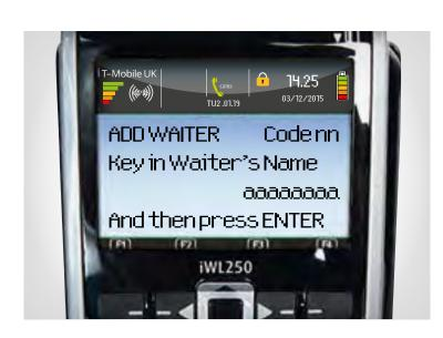
6 Your card machine will automatically allocate the next available waiter ID (this field is limited to 10 characters). Key in your waiter's name and press the
