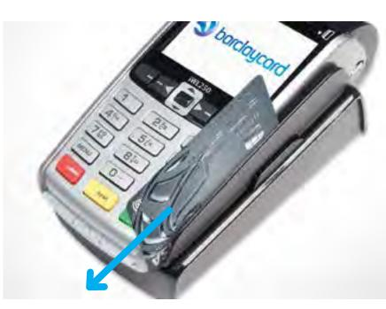
2 Swipe the customer's card with the magnetic stripe inserted into and facing the card machine.
