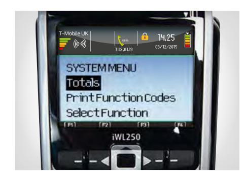
1 At the 'ready' prompt, press the button until the system menu is displayed and the 'totals' option is highlighted.
