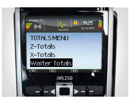
2 Using the arrow, highlight the 'waiter totals' option. Press the button.
