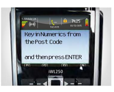
ask you to check the customer's address by entering the postcode. Enter only the numbers, for example if your postcode is NN4 7SG then enter '47'. Press the button.
