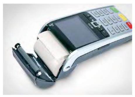
Peel away the end of the new roll. Leaving the end free, hold the till roll and carefully place into the printer compartment.
