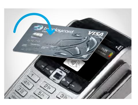
2 The cardholder should hold their card or contactless payment device against the display screen showing the contactless symbol (within 4cm).
