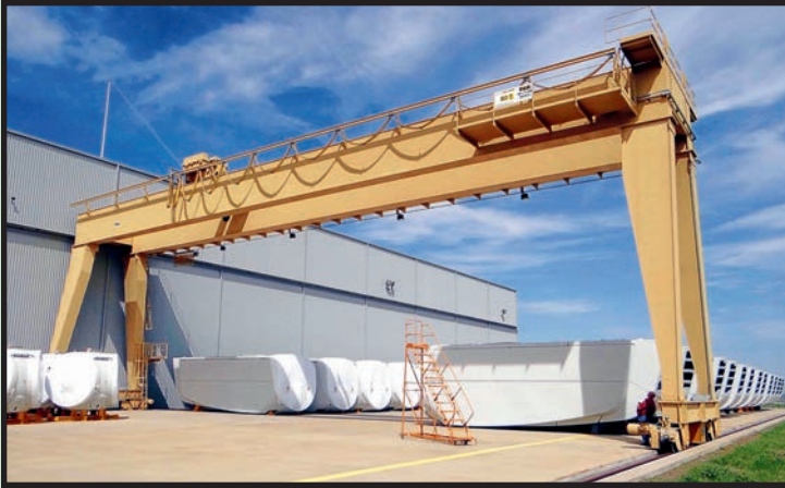
P&H 88 T. CAP. X 77' SPAN DOUBLE LEG GANTRY CRANE (SHOWN PRIOR TO DISASSEMBLY)
