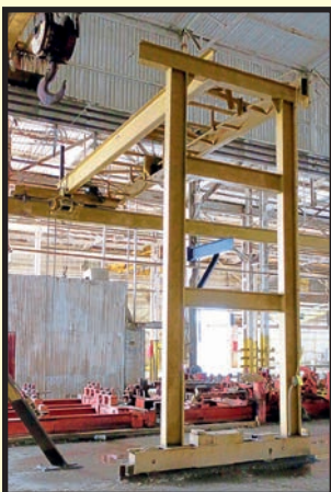
25' W. SINGLE LEG GANTRY CRANE
