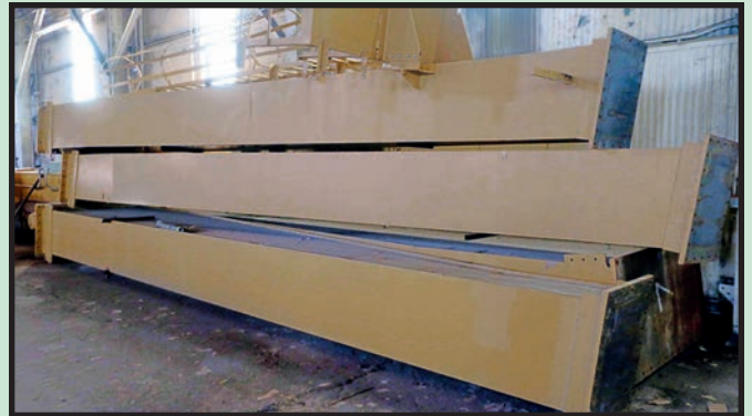
GAFFEY 30 T. CAP. DOUBLE LEG GANTRY CRANE UPRIGHTS
