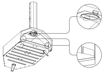
**Ceiling vent**: When this is closed, it will reduce air flow and allows hot air to gather inside the oven for longer.
