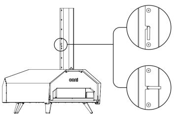
**Open (vertical position):** Maximum airflow encourages a hot burn for wood and charcoal.
