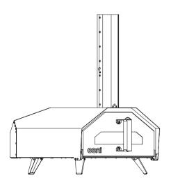
To close the **Door with Thermometer** Align the bottom edge hinges, raise the door until almost closed then lift and release on to the latch.
