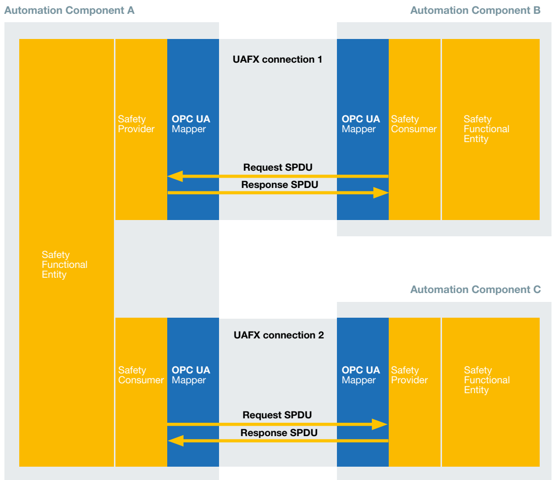
Figure 19: Safety connections between Automation Components
