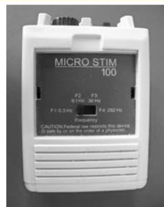
Figure 1: Phase one microcurrent machine using 4 basic Nogier frequencies.
