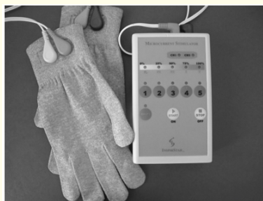
Figure 4: Phase two microcurrent machine customized able to program frequency pairs.
