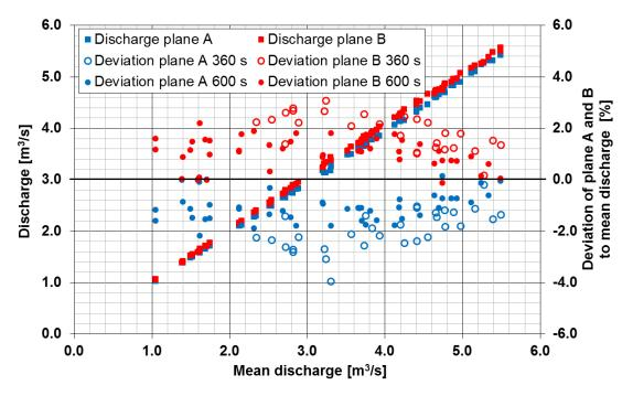
Figure 8. Discharge and deviation of planes A and B for all measuring points.
