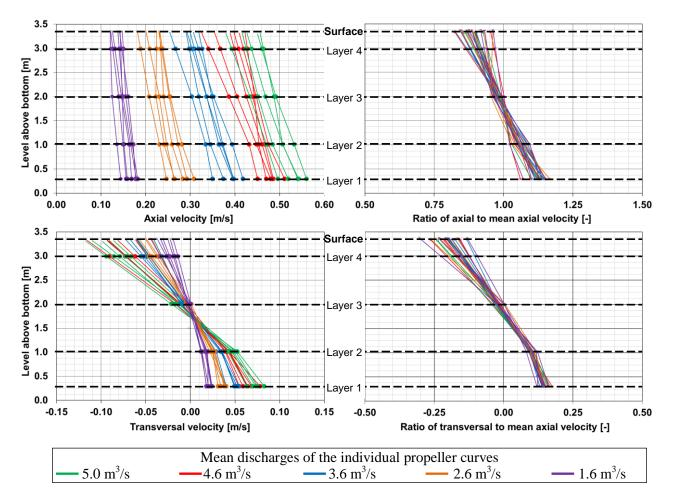
Figure 4. Measured axial and transversal velocity components with linearly extrapolated surface velocities.
