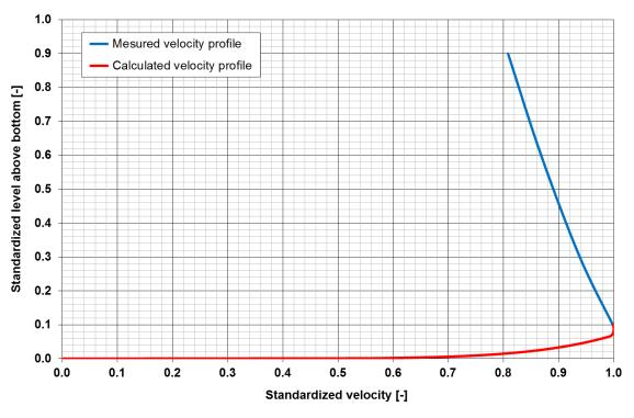
Figure 6. Extrapolation of the bottom axial velocity with  $K_{bot} = 0.9$ .
