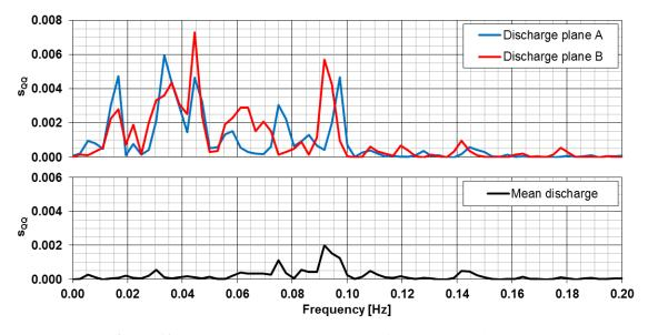
Figure 10. Auto power spectrum analysis for one measuring point.
