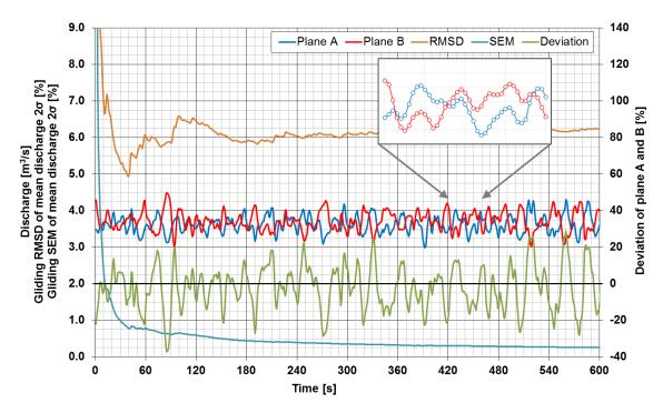
Figure 9. Discharge, statistics and deviation of planes A and B for one measuring point.
