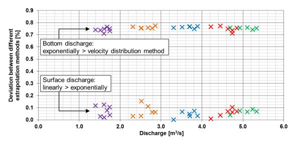
Figure 7. Influence of the extrapolation method for the surface and bottom velocities on the discharge.
