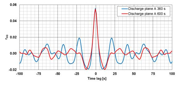
Figure 11. Auto correlation of the discharge in plane A for different acquisition durations.
