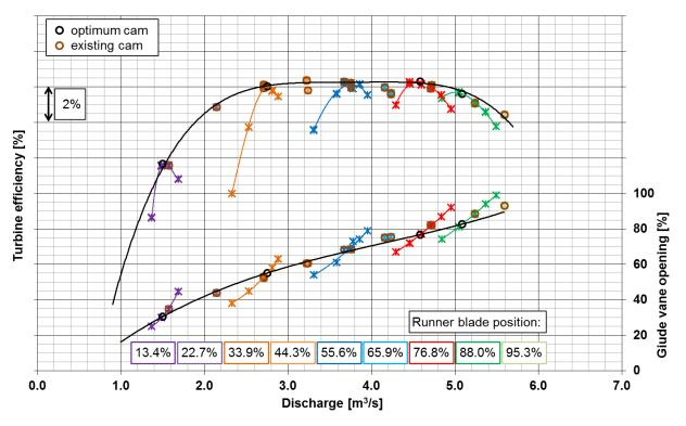
Figure 13. Turbine efficiency and cam correlation for MG 1 at the dotation HPP Pradella.
