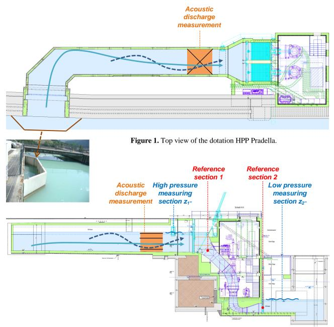
Figure 2. Side view of the dotation HPP Pradella with a schematic of the flow in the open channel.
