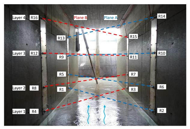
Figure 3. ATT installation within the rectangular open channel.
