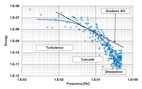
Figure 12. Example of turbulence spectra of measured axial velocity for one path.
