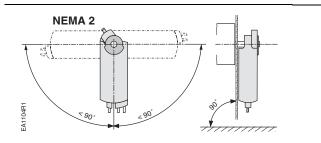
Figure 17. Acceptable NEMA 2, IP54 per EN 60 529 Mounting Positions.
