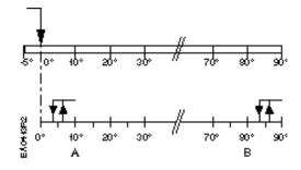
Actuator rotary range with the shaft adapter mounted at position "0".
