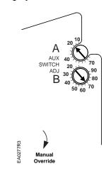
Figure 16. Dual Auxiliary Switch Dials.
