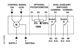
Figure 24. GCA13x, Floating Control.
