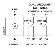
Figure 25. GCA22x, 2-Position Control.
