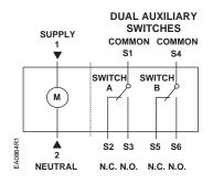
Figure 23. GCA12x, 2-Position Control.
