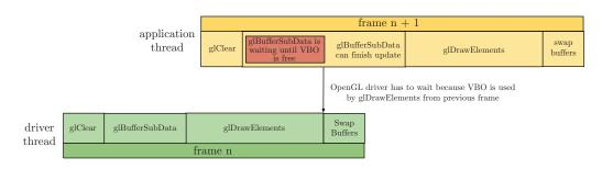
Figure 28.3. Implicit synchronization with glSubBufferData.
