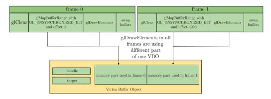
Figure 28.6. Possible usage of unsynchronized glMapBufferRange.
