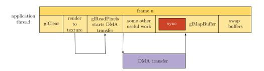
Figure 28.7. Asynchronous DMA transfer in download.
