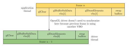
Figure 28.4. Avoiding implicit synchronizations with a round-robin chain.
