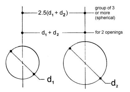
Furthermore, two openings in a group of three or more must have a minimum center distance equal to 2.5  $(d_1 + d_2)$  when in spherical shells or heads or  $(1 + 1.5 \cos \theta)(d_1 + d_2)$  when in cylinders or cones:
