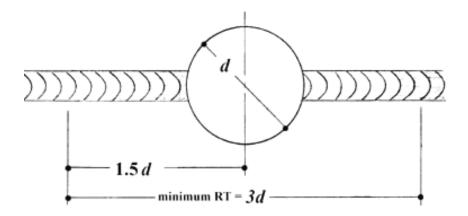
To be considered insignificant, an opening's edge cannot be closer than  $\frac{1}{2}$  inch to a nonradiographed joint unless the opening is made in plate > 1 $\frac{1}{2}$  inch thick. To remain insignificant, two or more inline openings located in a weld joint must meet the spacing requirements presented in UG-53.
