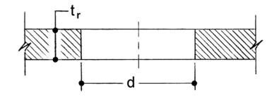
From here on, the nominal (or apparent) opening size will be designated by d, irrespective of its shape. The actual (Code defined) opening size will be designated d'; it is this latter value that must be used in the above formula.
