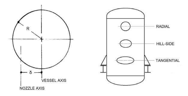
Openings are divided into the two broad classifications of radial or non-radial. The *Z* axis of a radial opening emanates from the center of the radius of curvature whose surface it penetrates. The best way to depict the various orientations is through the nozzle diagrams below. Nozzle is the term given by tank and pressure vessel designers to the connecting appurtenance which generally projects beyond the vessel's surface and terminates with a means of joining piping or equipment.
