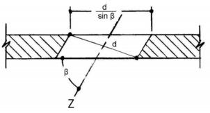
Like the circular hill-side and tangential, a circular inclined opening produces an elliptical shape.
