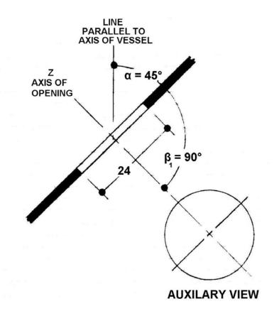
② Since  $\beta_2 > 45^\circ$ , the opening's Z axis is not parallel with the conical head's circumferential axis. This opening, whose axis is not parallel with either vessel axis, is an inclined opening with an inclination angle,
