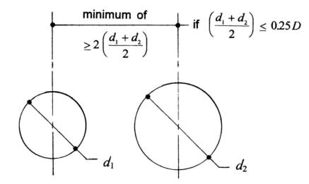
If the coefficient in the center-to-center distance equation above is < 2 but \$ 1.25, the 50% additional material rule can be applied to each opening, then summed, and distributed so that  $\frac{1}{2}$  of the total additional material is situated between the two. If openings are closer than
