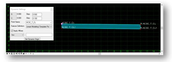
The **Point Name** can be keyed in or selected from the drop-down menu. When selected from the menu, the **Point Style** is automatically assigned for the point according to ODOT standards.
