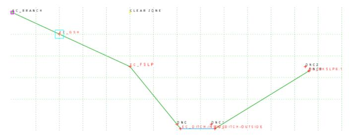
These templates have additional do not construct (DNC) points. These points are needed to set up the template to push the ditch to lower elevations in order to meet minimum ditch depths.
