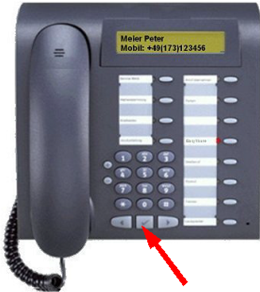
Figure 56: EasyLookup - Call the menu by pressing the application button on the device
