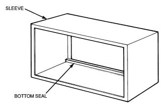
Fig. 7 — Remove Bottom Seal from GE Plastic Sleeve
