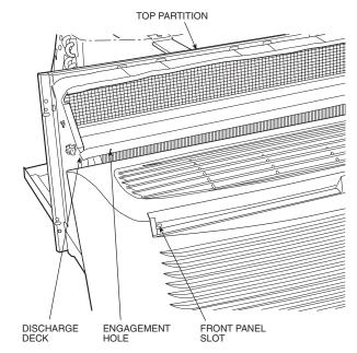
Fig. 4 — Front Panel Installation with Locking Feature
