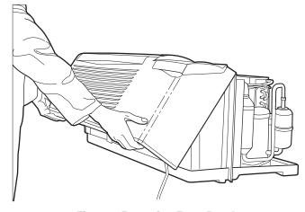
Fig. 2 — Removing Front Panel
