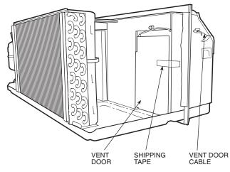
Fig. 9 — Location of Shipping Tape on Vent Door
