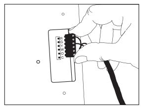
Fig. 14 — Terminal Connector Removal and Replacement
