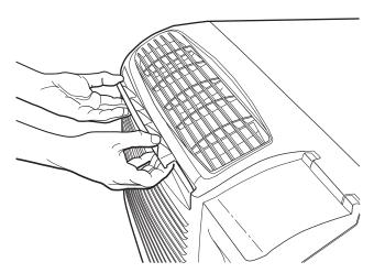
Fig. 19 — Indoor-Air Inlet Filter Removal
