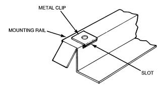
Fig. 6 — Remove Metal Clip on GE Metal Sleeve
