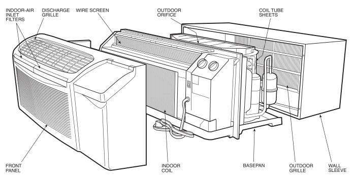
Fig. 8 — Unit Components
