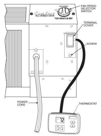
Fig. 12 — Control Box Terminal Cover
