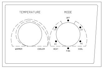
Fig. 17 — Standard Unit Controls
