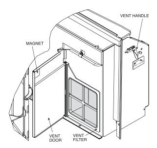
Fig. 20 — Outdoor Vent Filter (Left Side of Chassis)
