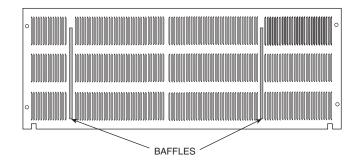
Fig. 5 — Remove Existing Outdoor Grille Baffles
