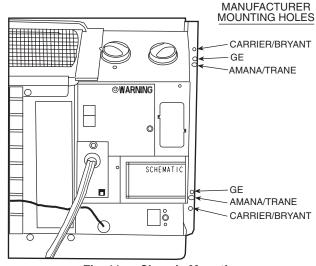
Fig. 11 — Chassis Mounting
