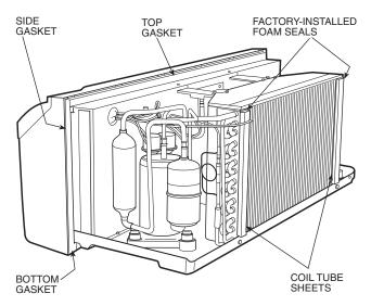
Fig. 10 — Unit Gaskets and Tube Sheets
