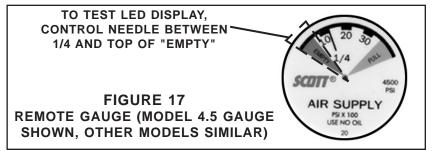
9. After verifying that the LED DISPLAY is functioning properly, vent the remaining residual air pressure from the system. The LED DISPLAY shall cease operation when the system pressure drops to zero.
