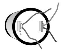
**5. Connect New Cluster** Connect new cluster to the using the same connections as the old cluster.
