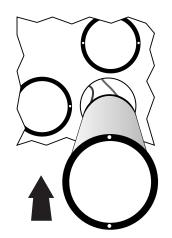
**6. Replace Cluster** Slide in new cluster with the holes lined up vertically (12 & 6 O'Clock).
