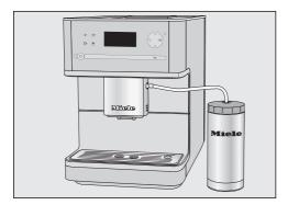
■ Place the milk flask beside the coffee machine. Connect the other end of the milk tube to the central spout.
