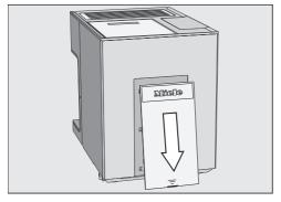
■ Slide the cover at the back of the coffee machine downwards.
