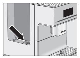
The water container filter is located underneath the water container.
