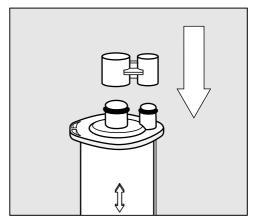
■ Seal the cartridge with the cap.
