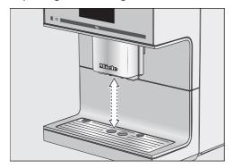
You can switch off spout adjustment. The central spout will then remain in the upper position while drinks are being made. When a maintenance programme is being carried out, the central spout will move to the height of the cleaning containers or into a maintenance position.
