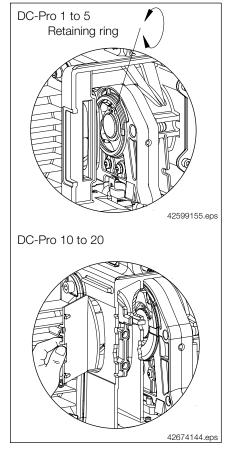
Fitting the chain anchorage DC-Pro 20, 2/1 reeving
