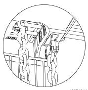
On reaching the permissible limit of chain wear, the chain set must be replaced (for determining the wear limit of the chain, see section 7.4).
