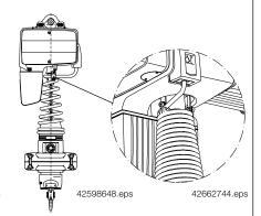
Disconnect helical cable, screws and pipe clamps from the adapter ring.
