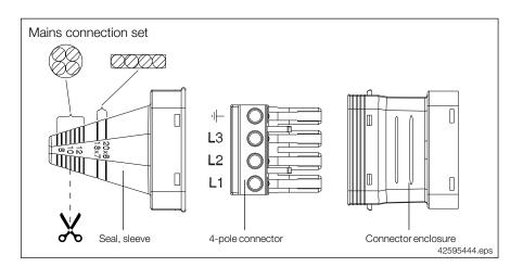
To connect the chain hoist to the power supply, the mains connection cable, the mains connection fuse links and the devices for disconnecting and switching the powerfeed must be available on site. For power supply, a 4-lead cable with an earth lead (PE), which complies with the table in section 2.4, is required.
