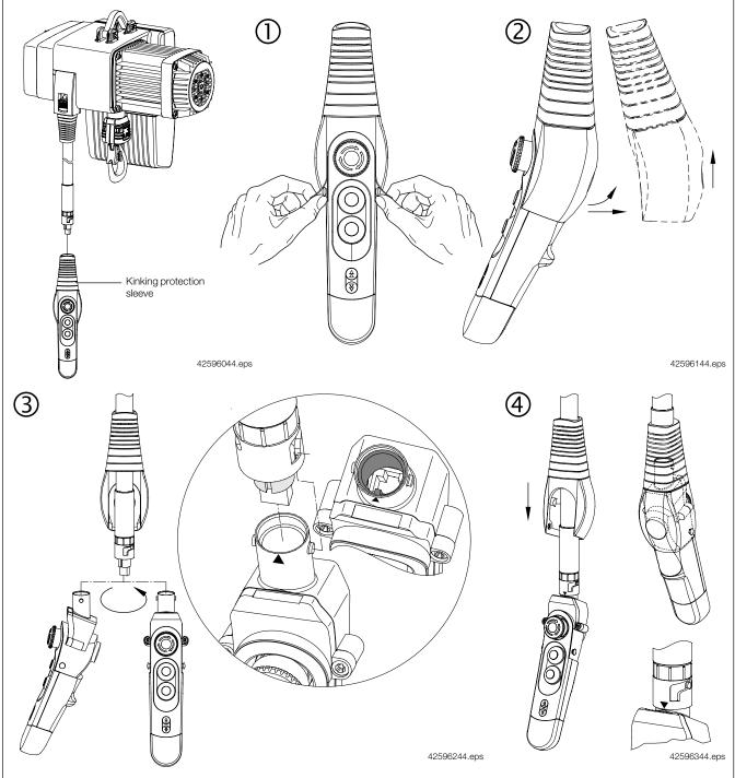
The control pendant is of plug-in design. Connect the DSC control pendant with the control cable and lock the connection with the bayonet lock.
