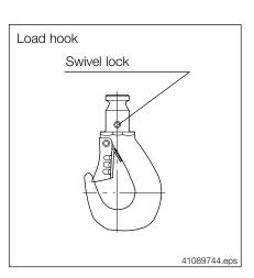
The swivel lock of the load handling attachment must not be removed.
