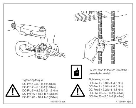
7.1.2 Replacing the bottom block for 2/1 reeving, DC-Pro 20
