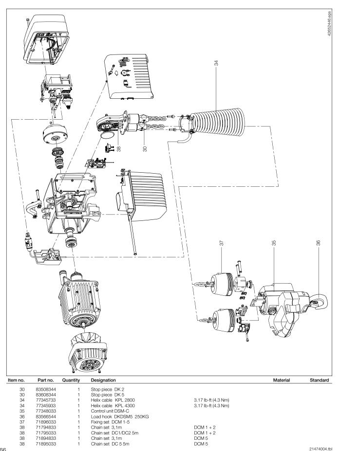
DEMAG Cranes & Components
