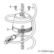
Undo cap screws (4), slide cap (5)
