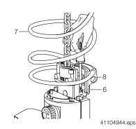
Undo flanged cable entry sleeve (6), remove helical cable (7). When fitting the new cable, seal by tightening the flanged cable entry sleeve with rubber seal.
