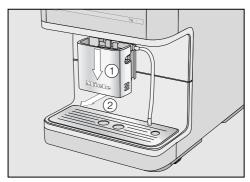
■ Push the main dispenser right down and remove the stainless steel cover by pulling it off towards you.
