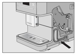
The milk tube for cartons and other suitable containers is located behind the appliance front.
