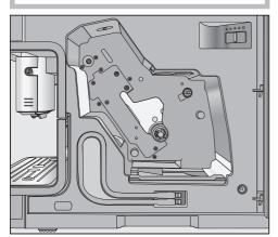
■ Clean the inside of the coffee machine. Make sure that the areas highlighted in the illustration are cleaned extremely carefully.
