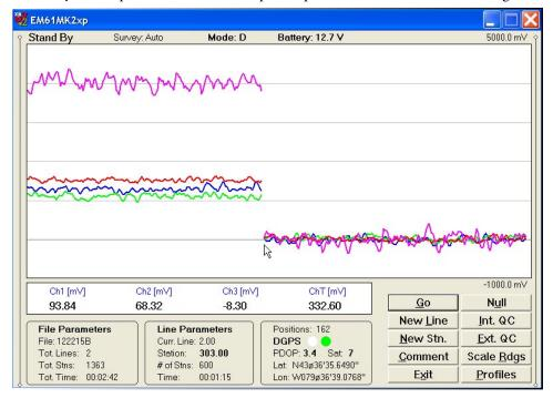
To ignore an entry and return to Stand By mode tap the **Cancel** (X) button or press **Esc** key, the dialog window will disappear and measurements can be continued.
