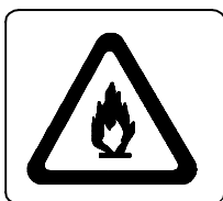
WARNING - Flammable liquid.
